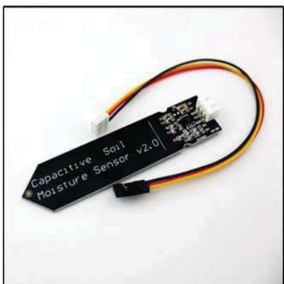
Fig.3 Capacitive soil moisture sensor
